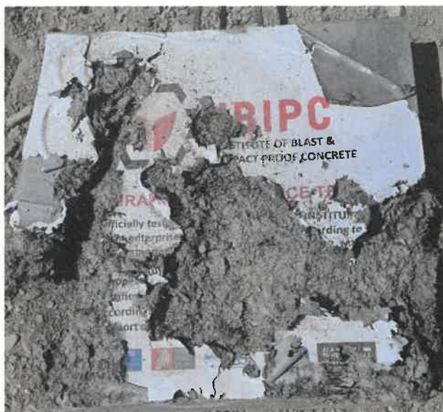
Obr. 8: Detail na čelní stranu vzorku 2 po testu Fig. 8: Detail on the front of the sample 2 after the test
